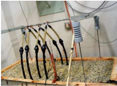
Set-up of the Multi-Stress Test developed by Cooper Power Systems to quantify long-term performance of connectors.
