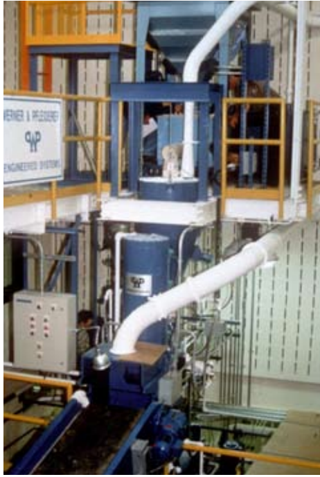
Computer-controlled mixer supplies EPDM insulation to all Cooper factories.
