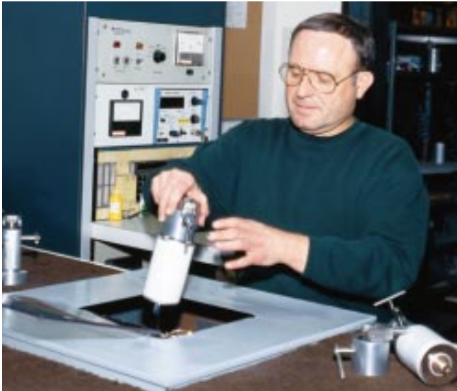
A Kyle vacuum interrupter is pressure tested.
