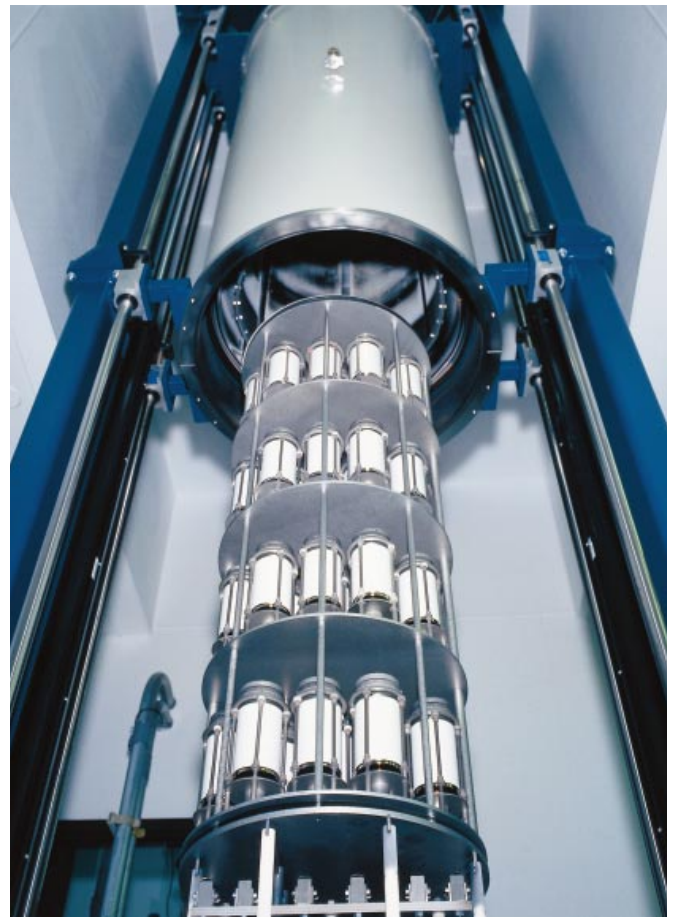
Vacuum interrupters are placed in high-vacuum brazing furnace.
