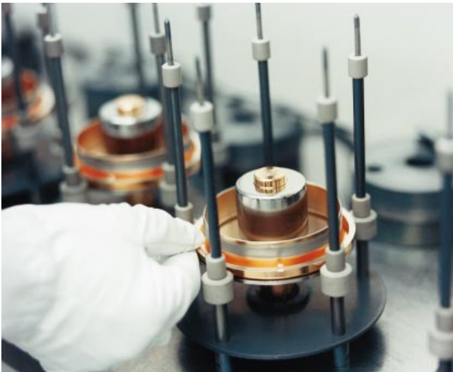
Vacuum interrupters are assembled in precision stainless steel fixtures.
