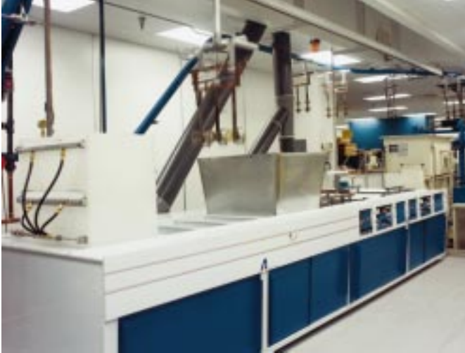
Electropolishing removes all contaminants from the interrupter contacts.
