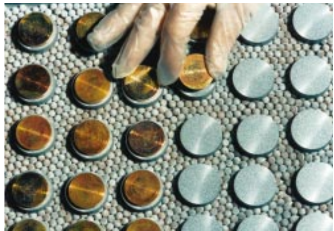
Copper placed onto chromium disks prior to contact infiltration.
